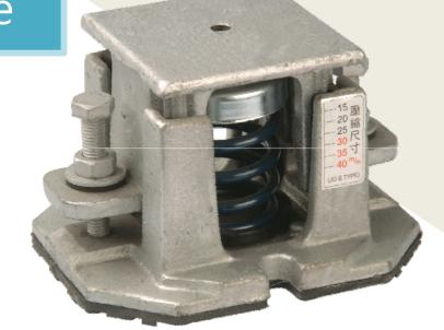
Adjust the adjustment nuts in the clockwise direction with 17mm open wrench to press down the spring (Fig 4).
